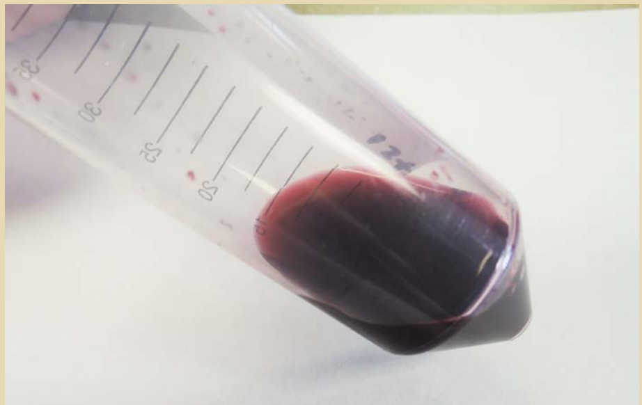
Gold nanoparticles synthesized according to our alkaline-based method. The average diameter is 30 nm.
