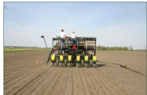
Figure 9-6. Six-row planter for corn and soybeans.
