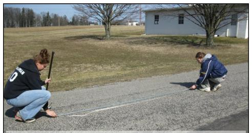
These frames can be made by one person but having a helper is best. Also, when using this method, the working surface must be smooth and firm. Layout a 10-ft section of pipe and tape measure side-by-side.
