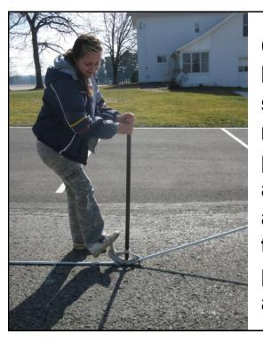
Continue the bend by the step-pull method. Use proper push and pull form and pace throughout the process to avoid injury.
