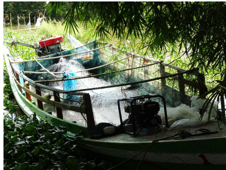
Specially modified fingerling transport boat with oxygenated 'live well'
