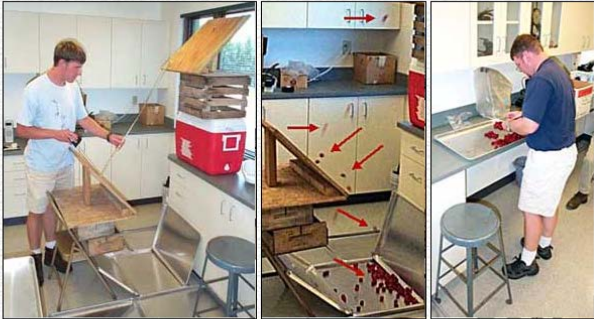
Figure 2. Simulated mechanical harvesting of fruit from GA growth regulator trials. The drop test approximates the fall of fruit from the tree onto belts from mechanical harvesters for laboratory analysis.
