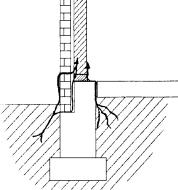
Figure 4.16. Poured foundation brick veneer (arrows indicate possible termite entry points).
