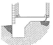
Figure 4.19. Completed treatment of monolithic slab—tile floor (dark shading shows areas treated).
