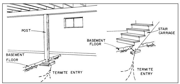
Figure 5.6. Wood post and basement steps extending through concrete (adapted from NPMA).
