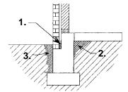
Figure 4.17. Completed treatment of poured foundation—brick veneer showing treatment of 1. the voids in the brick veneer, 2. the subslab soil area along the expansion joint, and 3. the outside perimeter of the building.
