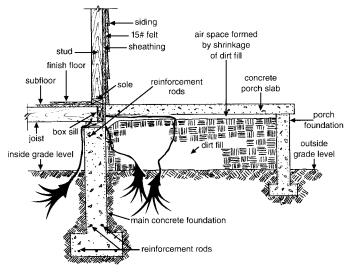
Figure 5.8. A common type of construction that involves a dirt-filled concrete porch attached to a frame house. Avenues of termite access are indicated by the heavy areas in the soil (NPMA).
