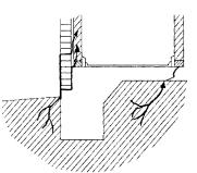
Figure 4.18. Monolithic slab tile floor (arrows indicate possible termite entry points).
