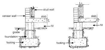
Figure 4.4. Suspended slab construction.
