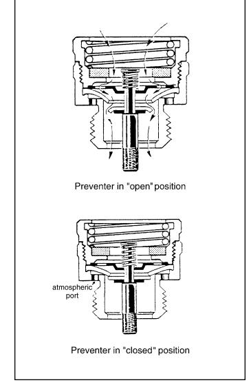
Figure 3.8. Backflow preventer in open and closed positions.
