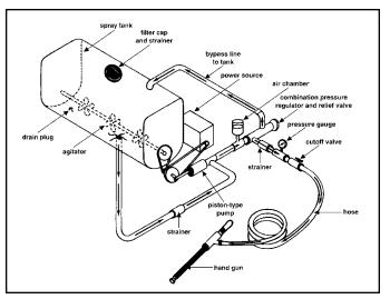
Figure 3.1. A schematic illustration of a simple power sprayer rig.
