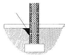
thor- Figure 4.8. Exterior slab treatment under (dark shading shows area treated).
