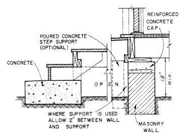
Figure 5.9. Construction of wooden steps of porch to prevent hidden termite entry (adapted from USDA).
