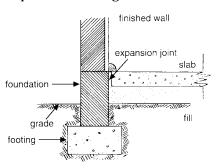
Figure 4.2. Floating slab construction.
