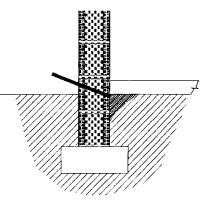
Figure 4.12. Short rodding (dark shading shows area treated).
