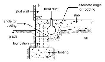
Figure 5.3. Rod treating adjacent to a perimeter heat duct.
