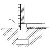
Figure 4.10. Treatment of brick or stone veneer (arrow points to treatment of void).
