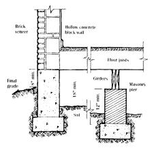
Figure 4.5. Crawl space construction.
