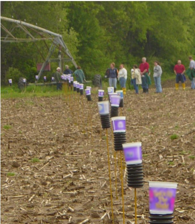
**Figure 7.** Catch can test to check uniformity of the center pivot system.
