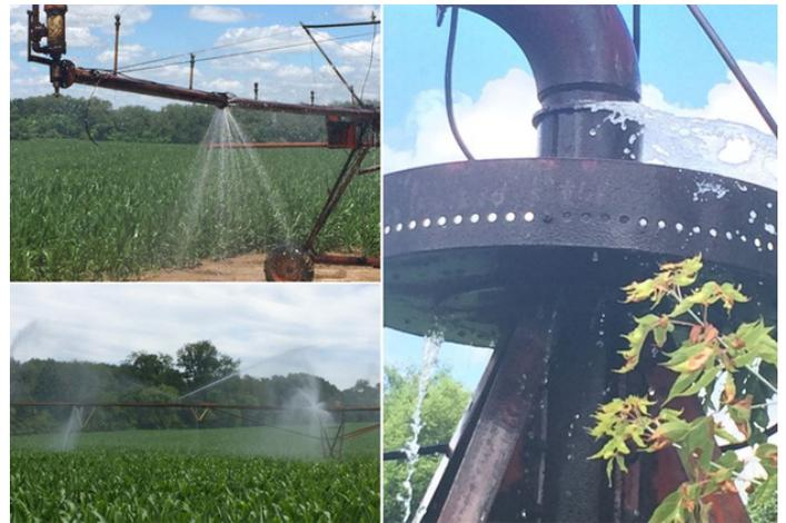
**Figure 9.** Pressurize the system and inspect for leaks, holes, and damaged sprinklers. Use a crayon mark, flag, or photo to identify the needed repair. The quicker the repair is made, the lower the crop damage incurred at the site.
