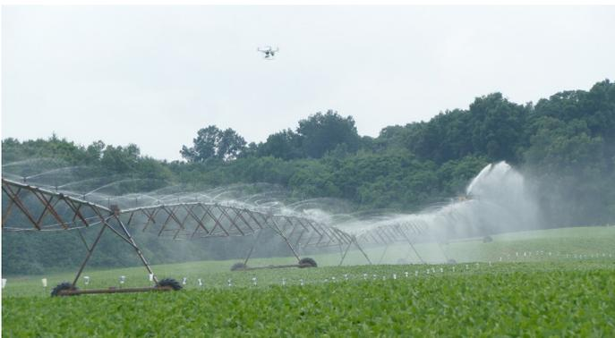
**Figure 8.** UAV to inspect the uniformity of the center pivot system (Photo Credit: Eric Anderson, MSU Extension Educator).
