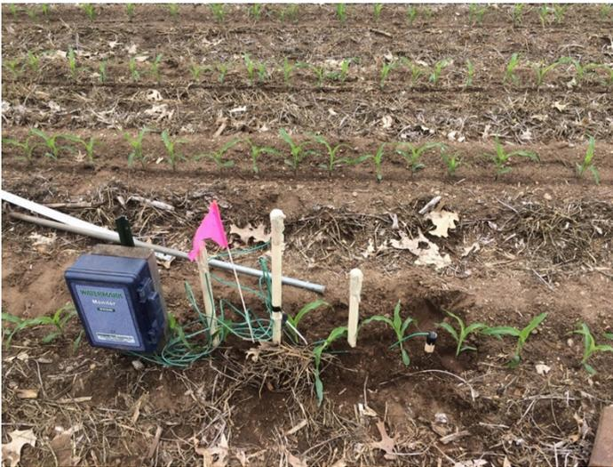
**Figure 2.** Soil moisture monitoring system in a seed corn field.
