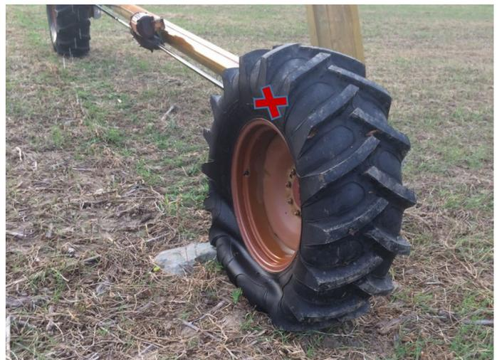
**Figure 11.** Tires are ruined quickly if run while low or flat. The pivot does not move normally with a flat tire, which may apply more water.
