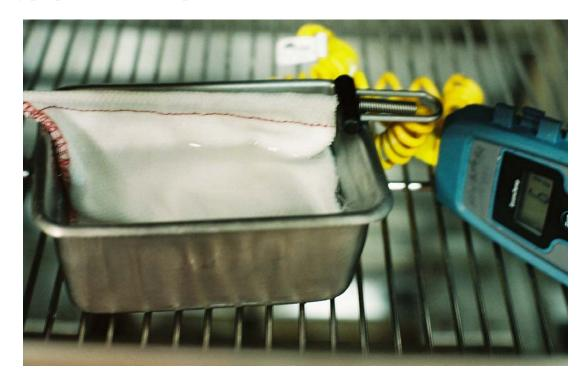
A wet-bulb probe needs to be placed close to the exhaust damper, and so that air can pass over the wet sock as it leaves the oven. Most engineers agree that the air at the exhaust damper is most representative of the condition of the air in the oven.
