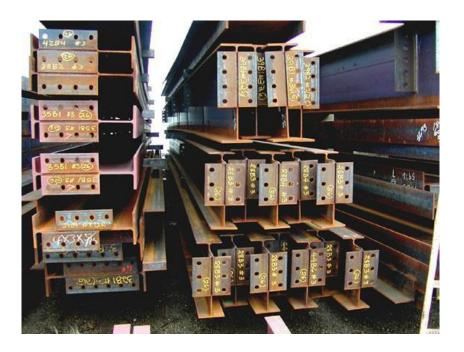
Fabricated beams ready to be shipped to construction site
