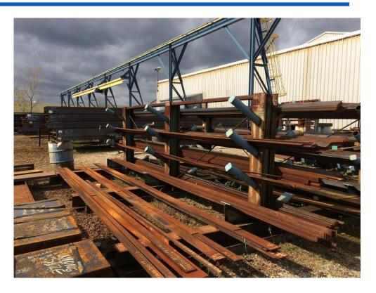
Racks used for storing plate and bar stock
