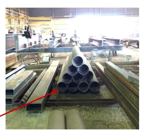
Round HSS shapes stored for fabrication —blocking is used to prevent shapes from rolling
