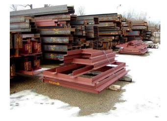
Fabricated beams and spandrel frames ready to be shipped to a construction site
