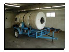
In-vessel Model 0824 (8' long, 36" diameter, 24  $yd^3$  capacity) has been used. The vessel consists of an insulated drum which is mounted on rotor casters. The drum is rotated by a chain drive approximately one complete rotation per 20 minutes. Materials are loaded and exit through ports at the ends of the drum. The drum is mounted at an incline to a steel frame resulting in the movement of the compost material from one end to the other as it rotates.
