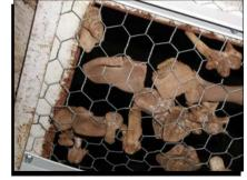
Screens were fabricated for the 3 exit doors using 1 inch chicken wire fencing. When the IV unit was emptied, the screen effectively prevented larger bones from being removed.
