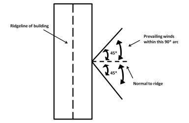
A barn or shed should be oriented to take advantage of prevailing winds. Positioning a barn in an elevated area with the stall windows facing the prevailing winds can facilitate a cross breeze during the hot summer months.
